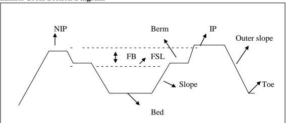
This diagram shows different locations of cross section of a channel, which are defined as under:
