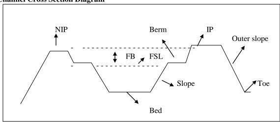
This diagram shows different locations of cross section of a channel, which are defined as under:
